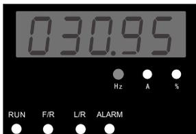
Operation status: running in forward rotation, frequency 30.95Hz.
