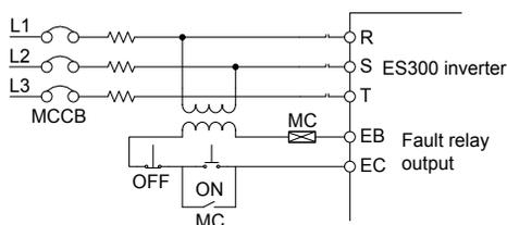
Fig 3-1 main circuit breaker wiring diagram
