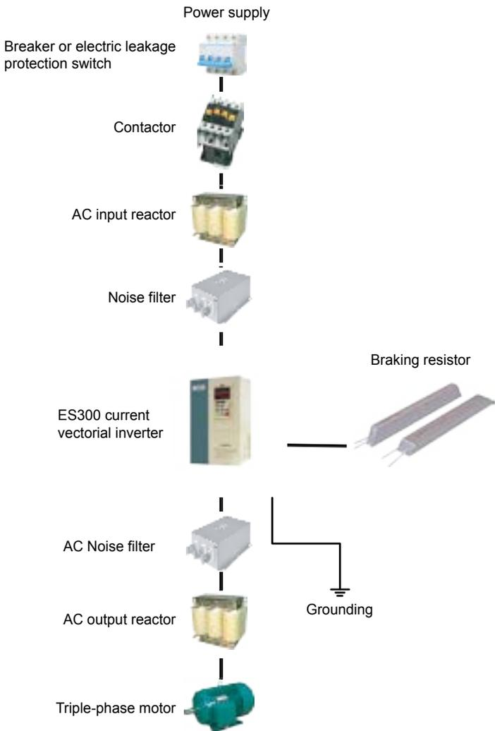
Fig 3-6 wiring diagram of inverter and peripheral equipment
