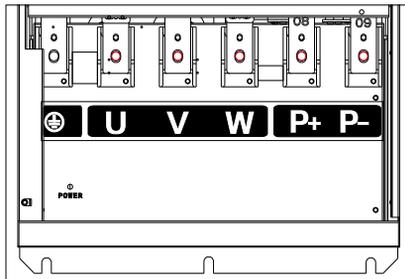
Fig 3-9 main circuit terminals diagram of ES300 132KW ~ 160KW
