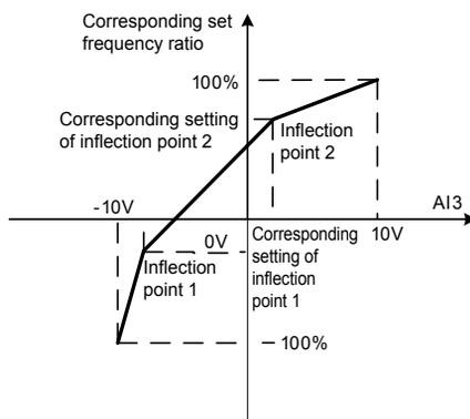
Fig 6-18 typical application case 3 of AI curve (4-points)
