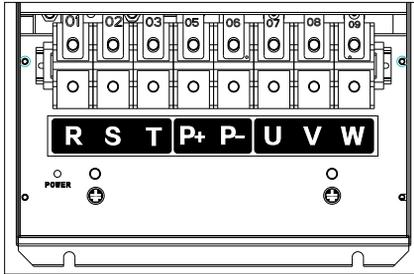
Fig 3-11 main circuit terminals diagram of ES300 75KW ~ 110KW
