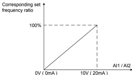
Fig 6-13 typical application 1 of AI curve (2-point) setting
