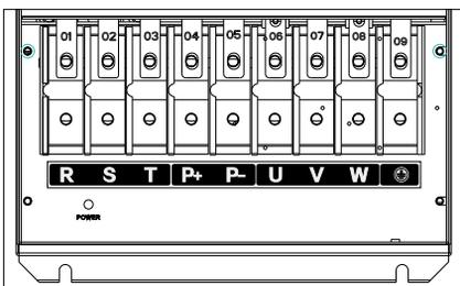
Fig 3-10 main circuit terminals diagram of ES300 45KW ~ 55KW
