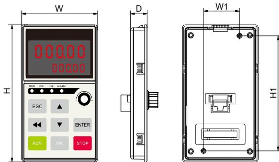
fig 2-4 keypad installation dimension diagram (unit: mm)
