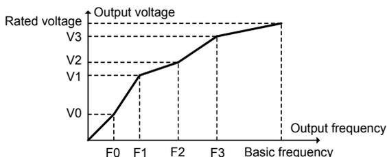
Fig 6-7 multi-points V/F curve diagram
