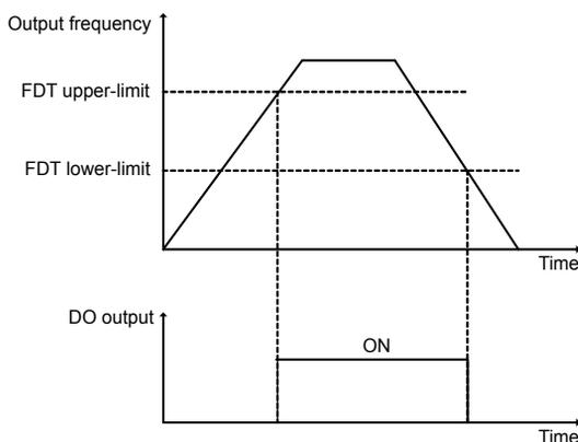
Fig 6-22 FDT frequency output level
