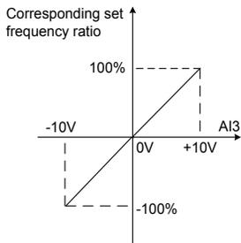
Fig 6-15 typical application 3 of AI curve (2-point) setting
