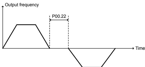
Fig 6-2 diagram of forward/reverse rotation dead-time
