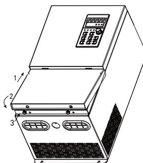
Fig 3-5 terminal cover installation
