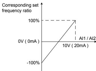
Fig 6-14 typical application 2 of AI curve (2-point) setting
