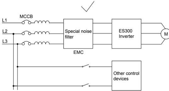
Fig 3-15 correct wiring of noise filter
