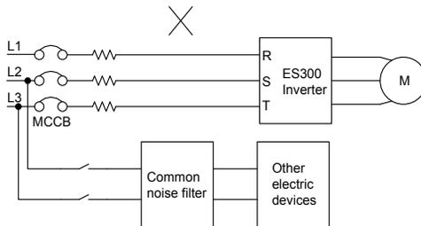
Fig 3-16 false wiring of noise filter
