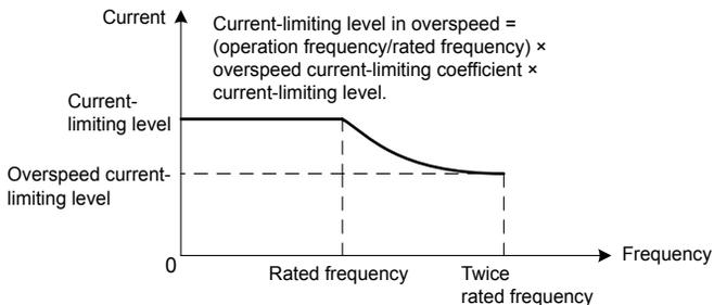
Fig 6-29 overspeed current-limiting level
