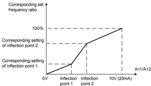
Fig 6-16 typical application case 1 of AI curve (4-points)
