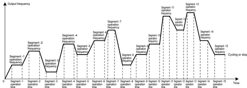
Fig 6-27 PLC multi-segment frequency operation
