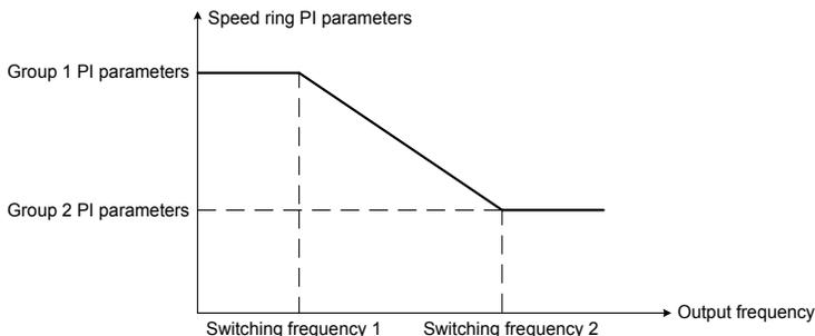
Fig 6-8 speed ring PI parameter switching diagram
