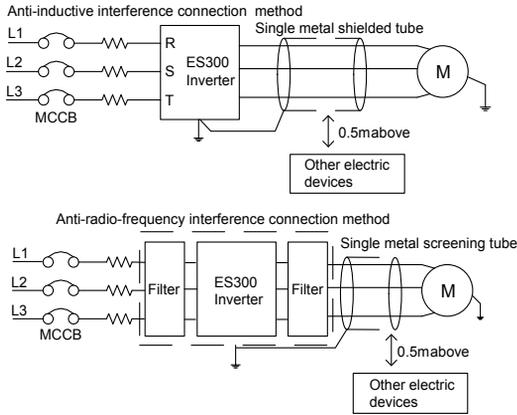
Fig 3-18 anti-interference installation wiring
