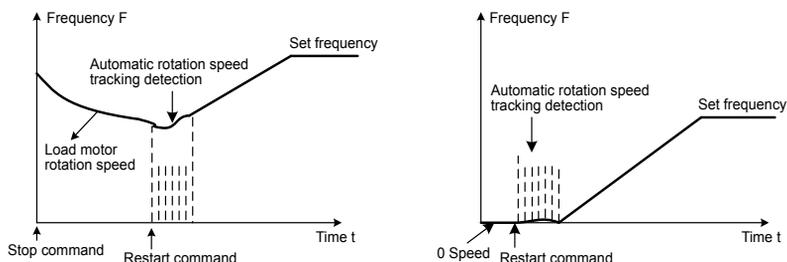
Fig 6-4 rotation speed tracking start diagram
