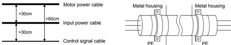
Fig 8-1 wiring requirement and shielded grounding way
