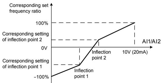
Fig 6-17 typical application case 2 of AI curve (4-points)
