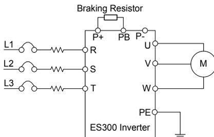
Fig 3-13 standard wiring diagram of main circuit
