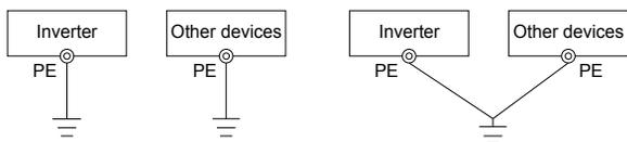
Correct grounding way of inverter and other devices
