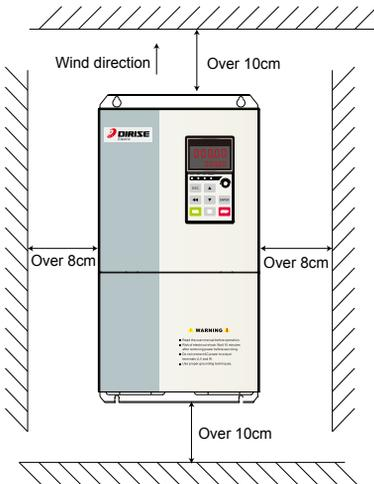
Fig 3-1 installation interval and distance diagram
