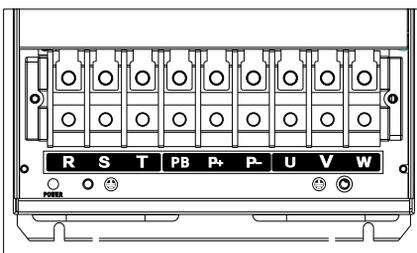
Fig 3-9 main circuit terminals diagram of ES300 30KW ~ 37KW ( Braking unit is selective )
