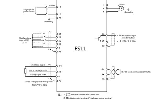
When multifunctional output terminals are connected to inductive load (e.g. relay coil), make sure to connect freewheel diode to both ends of load in parallel.
